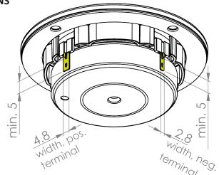
Thickness, both terminals: 0.5 mm Terminal plating: Gold
