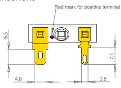
Thickness, both terminals: 0.5 mm Terminal plating: Gold
