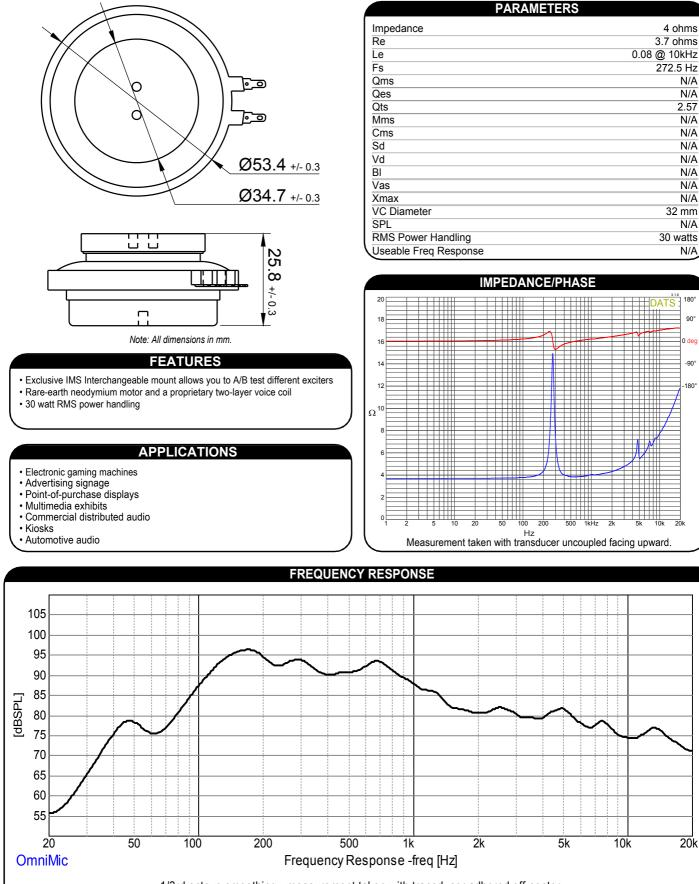
1/3rd octave smoothing - measurement taken with transducer adhered off-center on a 12" x 12" x 1/2" foam core board in an infinite baffle setup.
