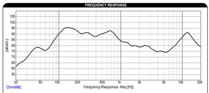
1/3rd octave smoothing - measurement taken with transducer adhered off-center on a 12" x 12" x  $\frac{1}{2}$ " foam core board in an infinite baffle setup.
